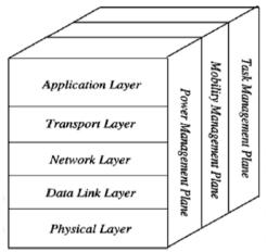
Figure: 2 .Wireless Sensor Network protocol stack
